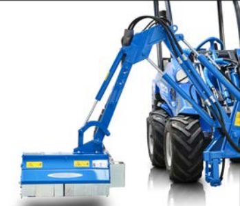
SIDE BOOM WITH FLAIL MOWER
