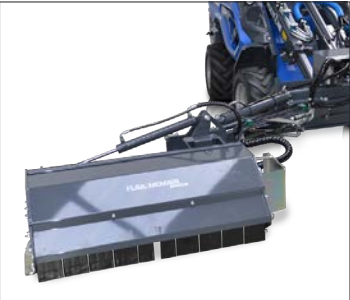
FLAIL MOWER WITH SIDE SHIFT
