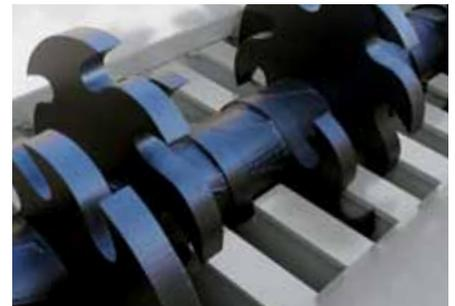
The knives are solidly welded onto the shafts; there are no bolts, bearings or adjustable parts anywhere in the cutting area, reducing servicing requirements.
